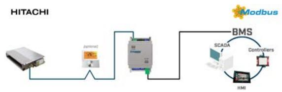
The AC interface has a compact design, is mounted on a DIN rail and requires no external power supply, as it is supplied via the air conditioner
